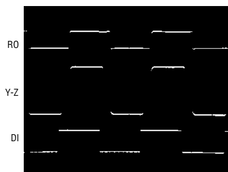
Normal Operation Waveforms at 250kbaud
