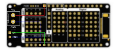
VIN: Connect to the VCC pin on the mainboard. The terminal is convenient for connecting the spiral battery. Note: When VIN is connected to an external power supply, do not connect the main control to other power supply or USB.
