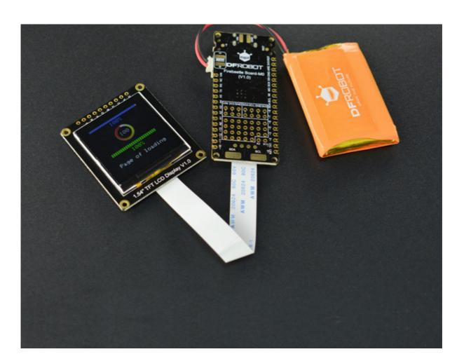
This interface is a DFRobot dedicated GDI, with 18pin-FPC cable connection and single wire connection to the screen, providing you with the simplest way to use the screen.
