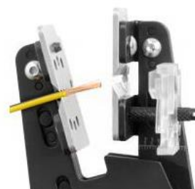
Automatic removal of insulation
