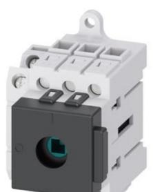
Switch disconnector 3LD3, main switch 3-polig, lu 40A operational switch at AC-23 A at 400 V 15,0 kW Distribution board mounting Base mounting with knob-operated mechanism with auxiliary 1NO+1NC
