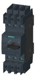
CIRCUIT-BREAKER SZ S00, FOR PLANT PROTECTION, WITH APPROBATION CIRCUIT-BREAKER UL 489. CSA C22.2 NO.5-02. A-RELEASE 0.16 A, N-RELEASE 2.1 A, SCREW CONNECTION, STANDARD SW. CAPACITY
