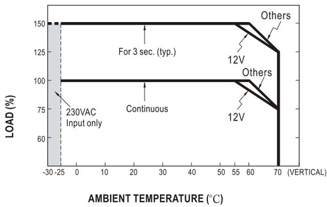
■ Output derating VS input voltage
