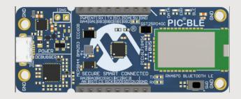
PIC-BLE Development Board (DT100112) AVR-BLE Development Board (DT100111)
