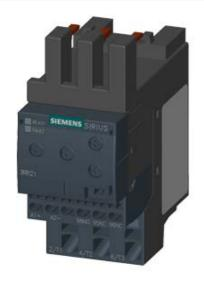
MONITORING RELAY ATTACHABLE TO CONTACTOR 3RT2. SIZE S0 BASIC, ANALOG ADJUSTABLE APPARENT CURRENT MONITORING 4 - 40A, 50-60 HZ, 2-PHASE SUPPLY 24 V AC/DC 1 CO CONTACT MONITORING FOR CURRENT OVERSHOOT/UNDERSHOOT PHASE FAILURE, WIRE BREAK WITH OR W/O ERROR LOG ON-DELAY 0-60 S SPURIOUS PEAK SUPPR.0-30 S SWITCHING HYSTERESIS 6% SPRING-LOADED CONNECTION
