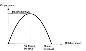
The torque vs. speed and output power curves depend on the supply voltage to the motor.
