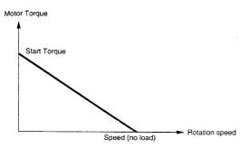
The curve for the output power of the motor is deduced from the graph of torque versus speed.
