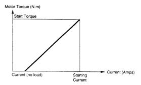
The graph for this relationship does not vary with the supply voltage of the motor. The end of the curve is extended in accordance with the torque and the start-up current.
