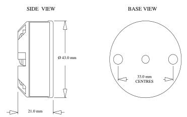
Fixing holes 2 x  $\emptyset$ 5.5 mm, Centre hole  $\emptyset$ 4.5 mm
