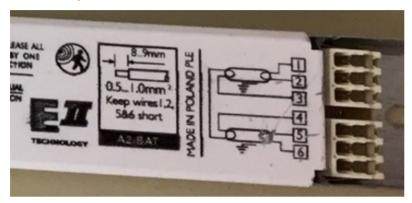
Step 2: Connect second fuse line to line "1" and "6"
