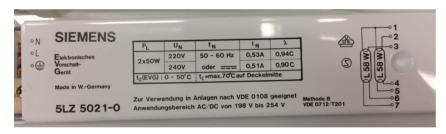
Step 2 Connect second fuse line to line "7" and "5"
