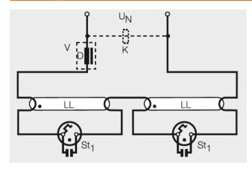
Remove wiring from CCG step by step and connect as described, if applicable remove compensation capacitor as well
