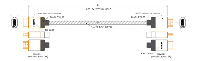
NOTE: E314459  $\,\%$  AWM 20276 80  $\,\%$  30V VW-1 HIGH SPEED HDMI $^{\oplus}$  CABLE WITH ETHERNET
