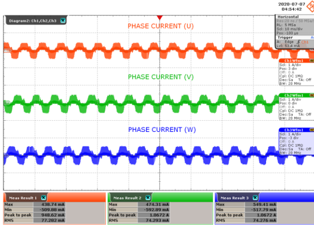
Figure 24 – Phase Current at Light Load.
