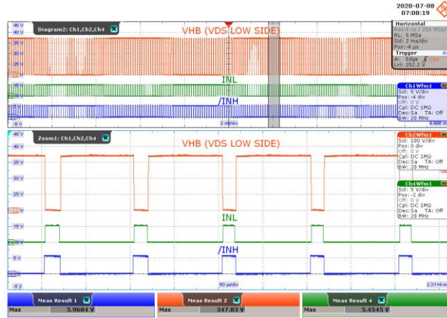
Figure 29 – INL and /INH Signal at 30 W Load. CH2: V_{HB\_PHASEW} , 100 V / div. CH4: V_{INL} , 5 V / div. CH1: V_{INH} , 5 V / div. Time Scale: 2 ms / div. Time Scale (Zoomed Area): 50 \mu s / div.
