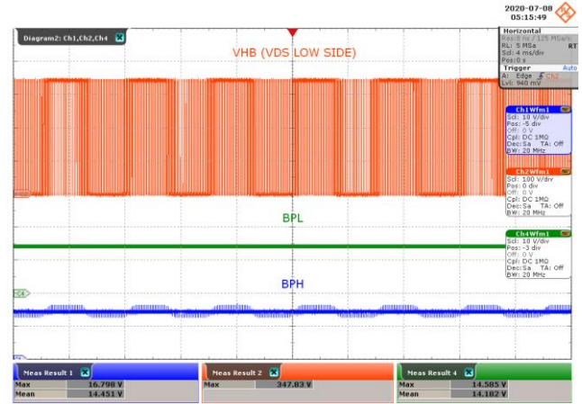
Figure 33 – BPL and BPH Signal at 30W Load. CH2: V_{HB\_PHASEW} , 100 V / div. CH4: V_{BPL} , 10 V / div. CH1: V_{BPH} , 10 V / div. Time Scale: 4 ms / div. BPL Average Voltage = 14.18 V. BPH Average Voltage = 14.45 V.
