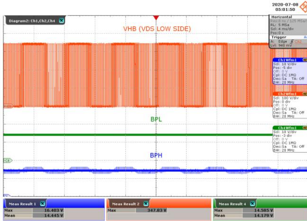
Figure 32 – BPL and BPH Signal at Light Load. CH2: V_{HB\_PHASEW} , 100 V / div. CH4: V_{BPL} , 10 V / div. CH1: V_{BPH} , 10 V / div. Time Scale: 4 ms / div. BPL Average Voltage = 14.17 V. BPH Average Voltage = 14.44 V.
