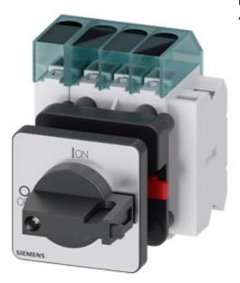
Switch disconnector 3LD3, main switch 3-polig + N, lu 40A operational switch at AC-23 A at 400 V 15,0 kW front mounted Base mounting with center-hole 22,5 mm knob-operated mechanism black  $48 \times 48$  mm with auxiliary 1NO+1NC
