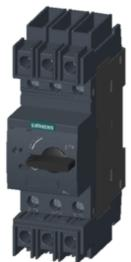
CIRCUIT-BREAKER SZ S0, FOR TRANSFORMER PROTECTION, WITH APPROBATION CIRCUIT-BREAKER UL 489. CSA C22.2 NO.5-02. A-RELEASE 22 A, N-RELEASE 364 A, SCREW CONNECTION, STANDARD SW. CAPACITY
