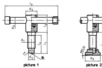
\* to ease assembly the DIN 6306 specification has been completed by r
