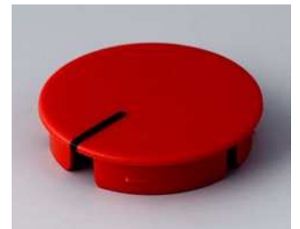
A4131102 Cover 31, with line ABS (UL 94 HB) red RAL F12/0-10
