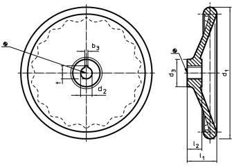
The orientation of the hub keyway may be different than shown in the drawing.
