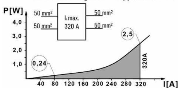
\*max. current at 2 x 50 mm<sup>2</sup> (according to IEC)
