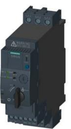
SIRIUS, COMPACT STARTER, DIRECT STARTER 690 V, 24 V AC/DC, 50 ... 60 HZ, 1 ... 4 A, IP20, CONNECTION MAIN CIRCUIT: SCREW TERMINAL, CONNECTION AUXILIARY CIRCUIT: SCREW TERMINAL
