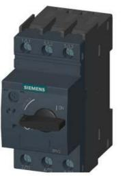
CIRCUIT-BREAKER SZ S0, FOR MOTOR PROTECTION, CLASS 10, A-RELEASE 27...32A, N-RELEASE 400A, SCREW CONNECTION, STANDARD SW. CAPACITY,
