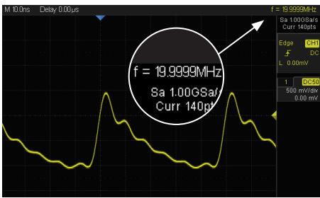
Built-in arbitrary waveform at 20 MHz, 300 MSa/s
