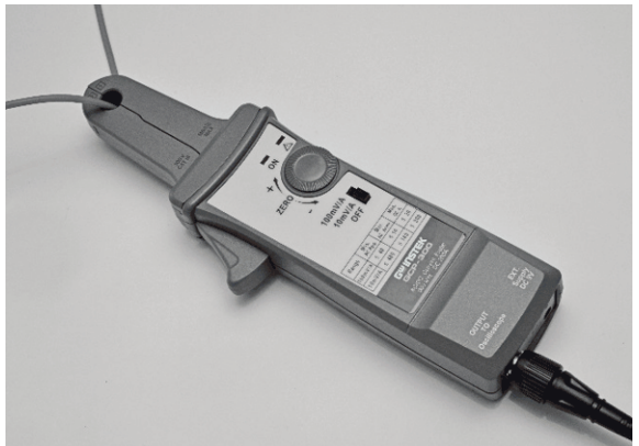
Figure 2. Connecting the GCP-300 current probe.
