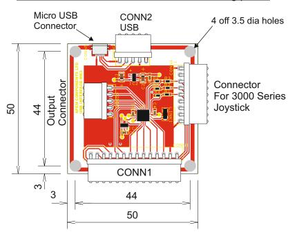
USB connection is made via either a 5 way 2.54mm pitch Molex® KK style header or a Micro USB type B socket on the board. A suitable USB cable (1.5m long) is included.
