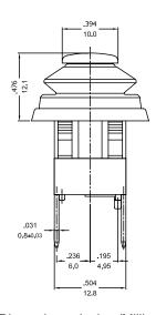
Dimensions : Inches/Millimetres Tolerances ±0.012"/0.3mm
