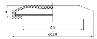
Used on dia. 19 mm flat actuator products to reach IP67 (not suitable for oil environments)
