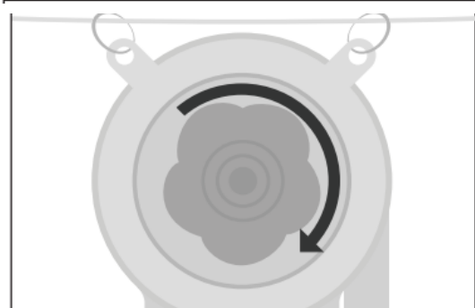
5. You can adjust the tensile level of the balancer by turning the rotator before use to avoid elastic fatigue which is caused by overload. Counter clockwise rotation for a tension increase; clockwise for a tension release.
