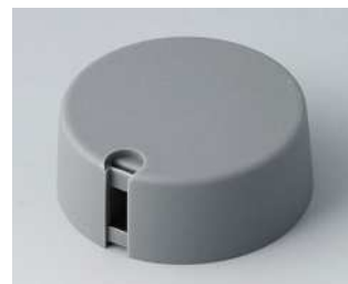
A1040048 TOP-KNOBS 40 PA 6 vulkan 40x16mm 4mm
