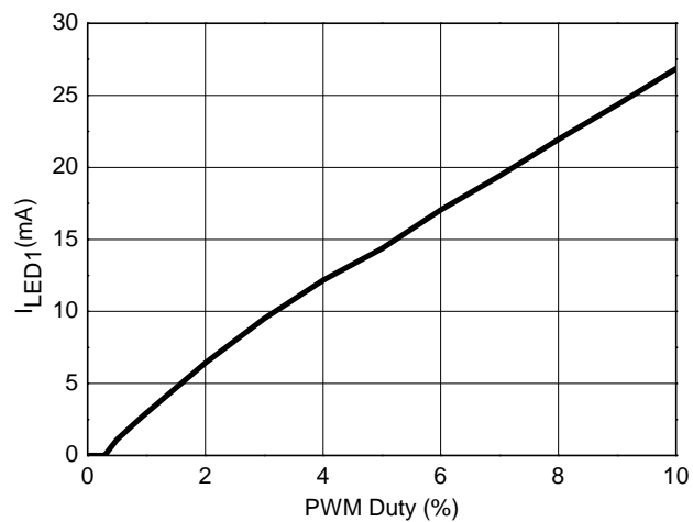
LED Current (AL1782) vs. PWM Duty (f=500Hz, 0~10%)
