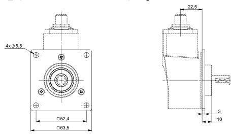
THK5\_14 Standard clamping, Connection BFR (M12), coupling 9445/016 mounted on the body
