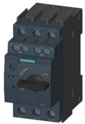
CIRCUIT-BREAKER SZ S00, FOR MOTOR PROTECTION, CLASS 10, A-REL. 0.7...1A, N-RELEASE 13A, SCREW CONNECTION, STANDARD SW. CAPACITY, W. TRANSVERSE AUX. SWITCH 1NO+1NC
