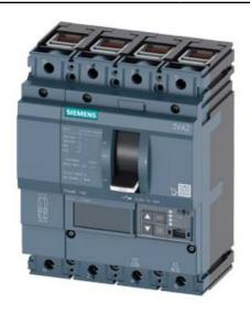
CIRCUIT BREAKER 3VA2 IEC FRAME 160 BREAKING CAPACITY CLASS M ICU=55KA @ 415 V 4POLE, LINE PROTECTION ETU860, LSIG, IN=160A OVERLOAD PROTECTION IR=64A ...160A SHORT CIRCUIT PROTECTION ISD=0,6..10X IN, II=1,5..10X IN NEUTRAL PROTECTION ADJUSTABLE (OFF, UPTO 100%) GROUNDFAULT, SWITCHABLE IG=0,2... 1 X IN, TG=0,050,8MS CABLE CONNECTION
