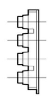
Actuating Force : 120 ±30 g Stroke : 2 ±0.5 mm Dimensions: Millimetres
