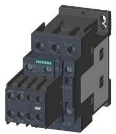
CONTACTOR, AC-3, 18.5KW/400V, 2NO+2NC, AC 110V 50HZ, 3-POLE, SZ S0 SCREW TERMINAL REMOVABLE AUX. SWITCH
