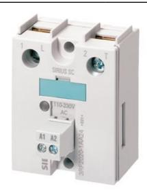
SEMICONDUCTOR RELAY 3RF2, 1-PH. WIDTH 45 MM, 70 A 48-600V / 4-30V DC SCREW CONNECTION BLOCKING VOLTAGE 1200V
