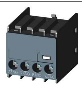
AUX.SWITCH BLOCK,FRONT,1NO+1NC, CURR.PATH:1NO, 1NC, CONN.F.BE., F. CONT. RELAYS A. MOTOR CONT., 3RT2 SCREW TERMINAL 73 / 74, 81 / 82
