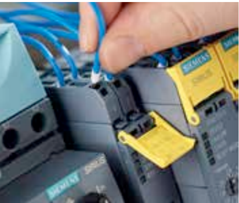
Terminals with optimized working angles: Cable routing and terminal operation occur from the same direction and are clearly visible during wiring. Labeled hinged covers facilitate the assignment of connections.
