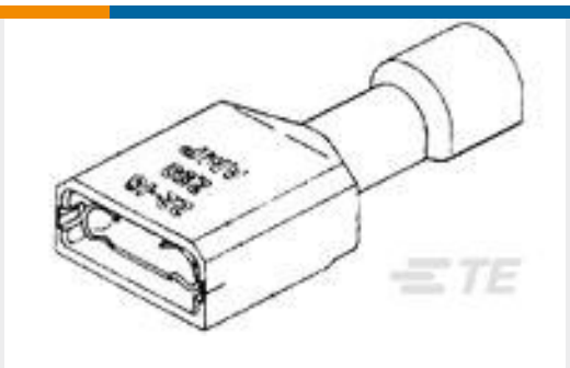
TE Part #2-520080-2 ULTRA-FAST .110/.125 ASY REC 22-18 TPBR
