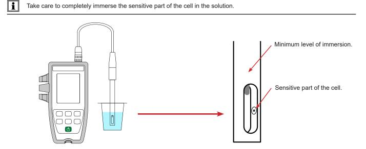
The cell provided with the instrument has an integrated temperature sensor. There is therefore no need to measure the temperature of the solution.
