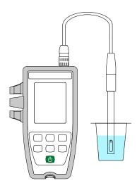
The instrument displays the measurement at the chosen reference temperature (20 or 25°C). Wait for it to stabilize before reading it on the instrument's display unit.
