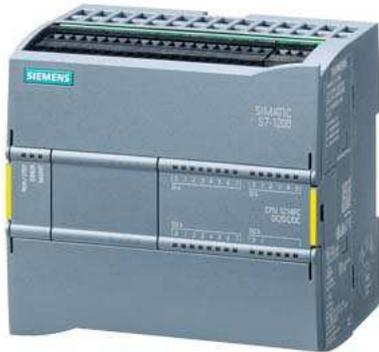
SIMATIC S7-1200F, CPU 1214 FC, Kompakt-CPU, DC/DC/DC, onboard I/O: 14 DI DC 24V; 10 DO 24V DC; 2 AI 0-10V DC, Stromversorgung: DC 20,4-28,8V DC, Programm-/Datenspeicher 125 KB
