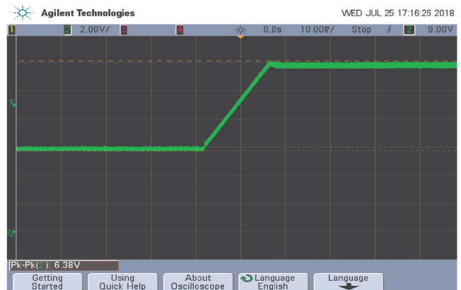
Figure 25 Output Pre-bias start-up Vin=48V, Iout = 0A, Cload = 10000µF, Ta = 25°C, Pre-bias Voltage = 9.6V
