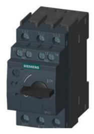
CIRCUIT-BREAKER SZ S00, FOR MOTOR PROTECTION, CLASS 10, A-REL. 1.4...2A, N-RELEASE 26A, SCREW CONNECTION, STANDARD SW. CAPACITY, W. TRANSVERSE AUX. SWITCH 1NO+1NC
