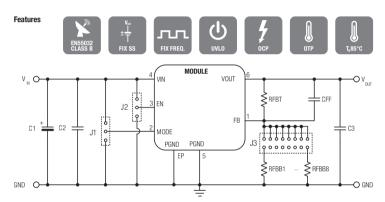
The additional aluminum polymer capacitor C1 is only for evaluation board protection purposes. It is mounted at the termination of the supply line and provides slight damping of possible oscillations of the series resonance circuit represented by the inductance of the supply line and the input capacitance. It is not essential for operation.
