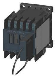
CONTACTOR FOR RAIL, AC-3, 5.5KW 400V, DC 24V, 0.7...1.25\*US, W. SUPPRESSOR DIODE INTEGRATED, 3-POLE, SIZE S00, SPRING-LOADED CONNECTION SPRING-LOADED TERMINAL
