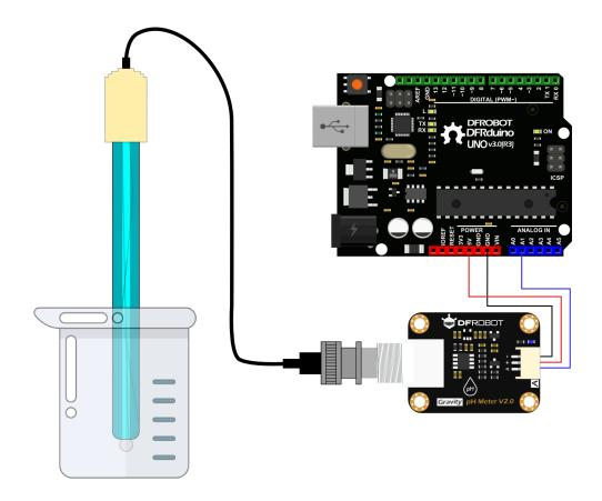
Arduino Connection Diagram
