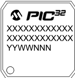
100-Lead TQFP (14x14x1 mm)
