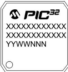
100-Lead TQFP (12x12x1 mm)
