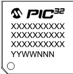
64-Lead TQFP (10x10x1 mm)
