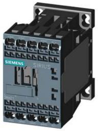
COUPLING CONTACTOR RELAY RAIL, 4NO, DC 24V, 0,7...1,25\*US, VARISTOR INTEGRATED, SZ S00, SPRING-LOADED TERMINAL
