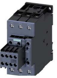
CONTACTOR,AC3:30KW/400V, 2NO+2NC,110VAC 50HZ/120V 60HZ, 3-POLE, SIZE S2, SCREW TERMINAL
