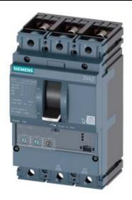
CIRCUIT BREAKER 3VA2 IEC FRAME 160 BREAKING CAPACITY CLASS H ICU=85KA @ 415 V 3POLE, LINE PROTECTION ETU320, LI, IN=25A OVERLOAD PROTECTION IR=10A ...25A SHORT CIRCUIT PROTECTION II=12 X IN BUSBAR CONNECTION
