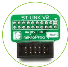
Figure 4-11: mikroProg™ to ST-LINK™ V2 adapter
